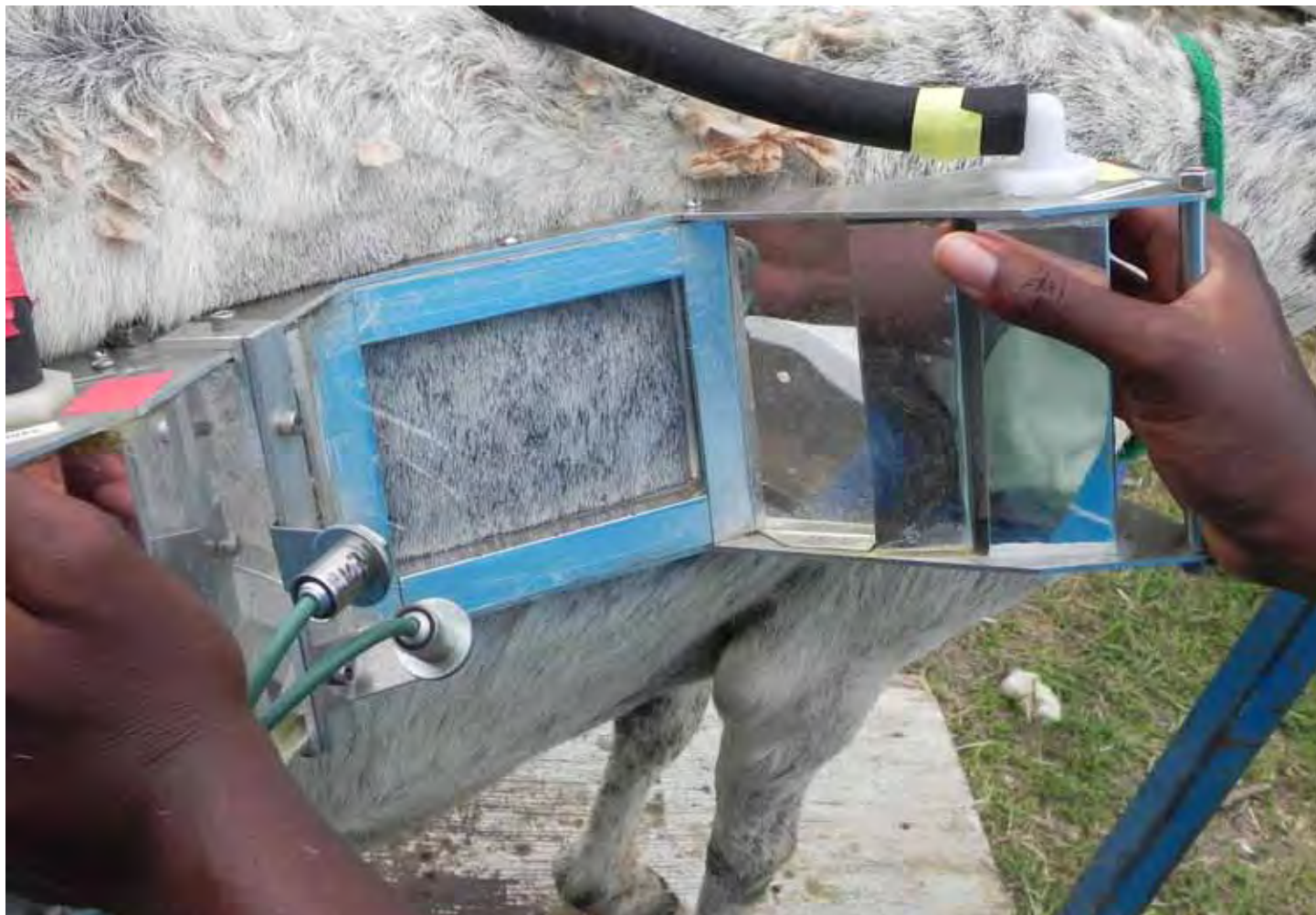
The sweating rate monitor (aka Bovine Evapometer) being used over the shaved area of a Dorper x St. Croix White ewe.
